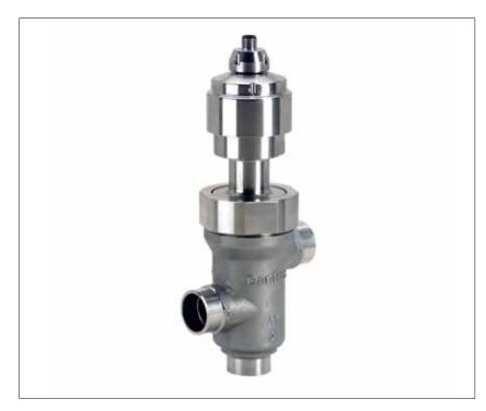
The CTR is an electrically operated 3-way valve designed specifically for operation in  $CO_2$  systems with heat reclaim. CTR is designed to allow full proportional control of the surplus heat from compressor pack into the heat exchanger of transcritical heat reclaim solutions.
